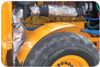
Top Photo: Removable Insulation Blankets on Vehicle Exhaust Piping
