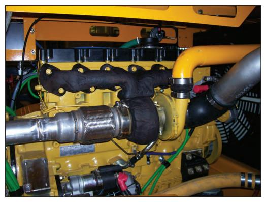
Over the last several years, rigid thermal coatings such as Firwin's HC, have found wider application in stationary and mobile engine systems.
