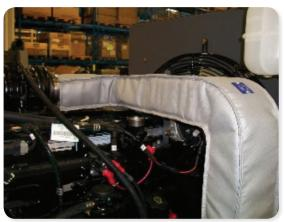
The configuration of exhaust piping, bends, elbows, etc., can significantly impact how heat flows through exhaust systems. Through the use of heat flow analysis systems, a more accurate assessment of real-world conditions can be made, which can affect the type and configuration of thermal insulation selected.
