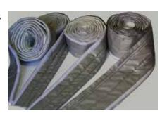
removable insulation blankets. The product features a silicone coated fiberglass outer cover, similar to Firwin's standard removable insulation blankets. Underneath is either ¼", ½", or 1" fiberglass insulation. Velcro hook and loop strips line either side of the T-Wrap™ for easy fastening and removal.
