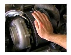
Users of removable insulation blankets often would like to know what the outside, or cold surface, temperature will be once the insulation blankets are installed on their system. This is especially true when personnel safety is of concern — the surface temperature of the blankets must be below a certain level to be considered safe for personnel working in the area.
