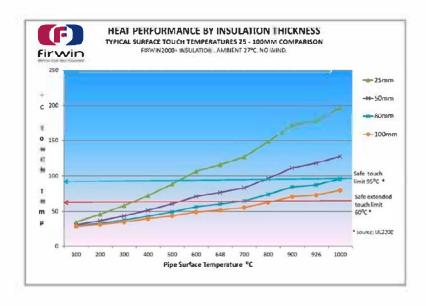
of how the outside surface blanket temperature will be affected by various material and thickness combinations", added Brett.
