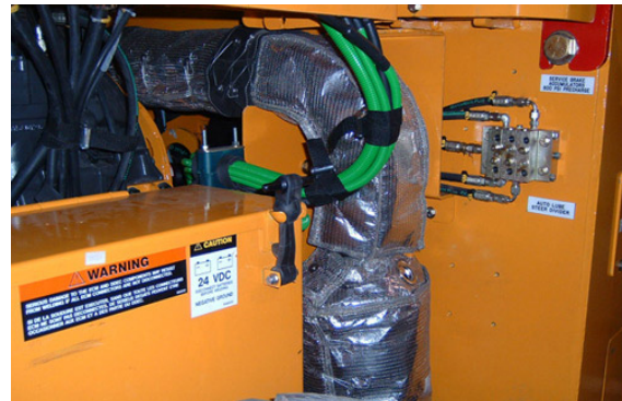
MineWrap™ Mark III blanket with reinforced outer liner
