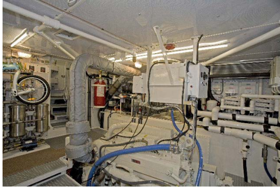
Engine room for Custom Steel '82 - Firwin Insulation Blankets on exhaust piping of twin Cummins engines
