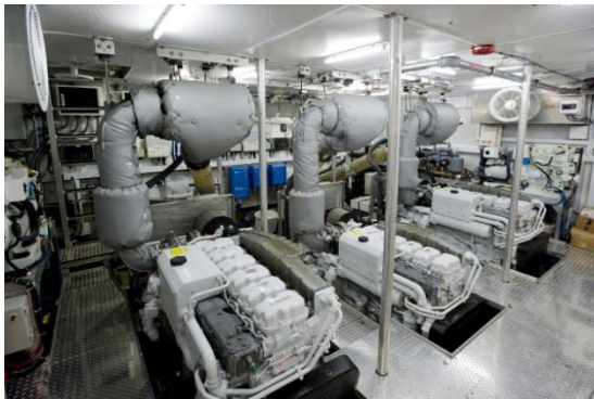
Engine room of Boundless '90 - Firwin blankets on mufflers and exhaust piping for three 720hp Yanmar Engines
