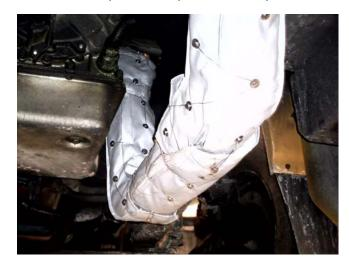
When the busses start rolling, take a peek at the exhaust. You just might see a Firwin insulation blanket along with a Ward Clean Air Filter helping to keep the air clean and safe for everyone.
