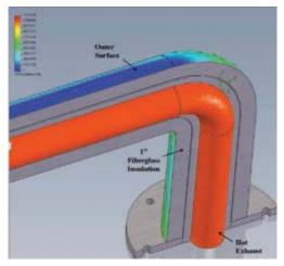
The configuration of exhaust piping, bends, elbows, etc., can significantly impact how heat flows through exhaust systems. Through the use of heat flow analysis systems, a more accurate assessment of real-world conditions can be made, which can affect the type and configuration of thermal insulation selected.
