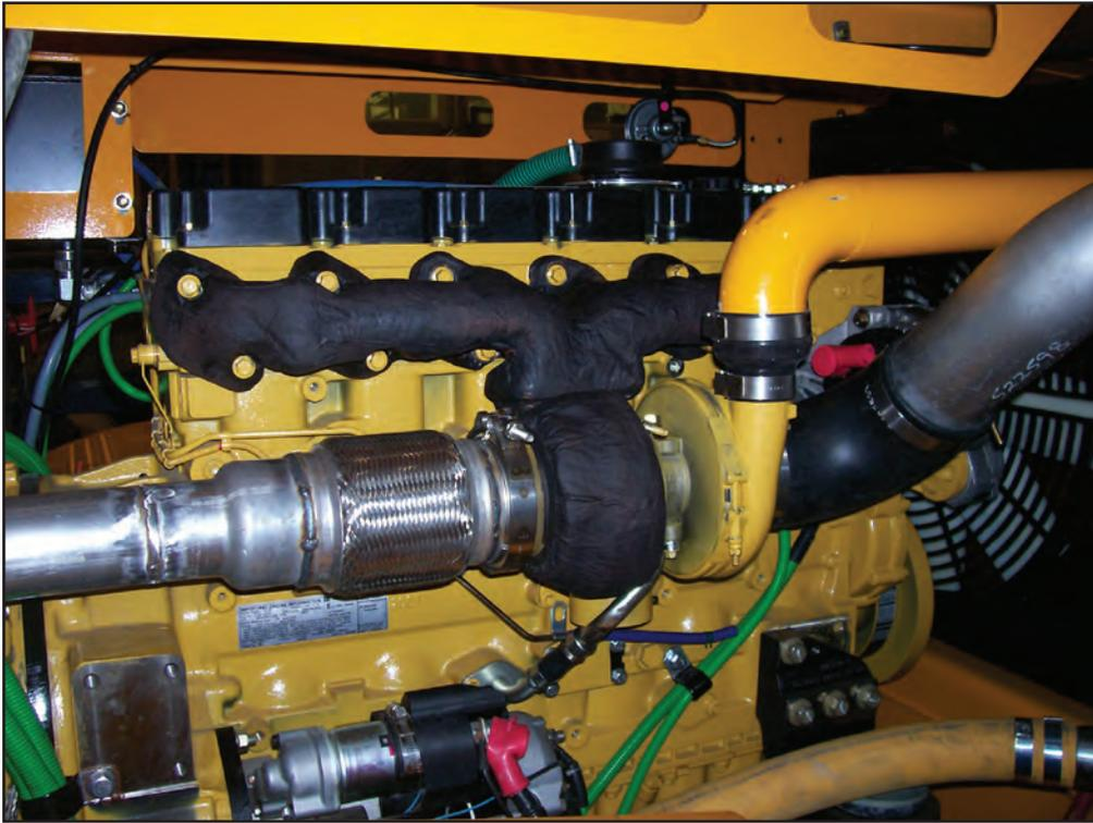
Over the last several years, rigid thermal coatings such as Firwin's HC, have found wider application in stationary and mobile engine systems.
