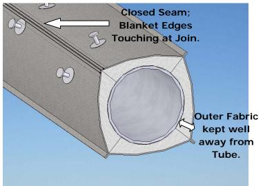
where the upper insulation blanket can cause a heat increase on the outer surface of the inner blanket. These outer fabrics, although rated for high temperature applications, are typically not designed to withstand temperatures greater than 500°F (260°C). If exposed to higher temperatures, either via direct contact with the exhaust piping, or via the heat generated by overlapping blankets, these outer fabrics can become heat-damaged and brittle, and possibly give off smoke.
